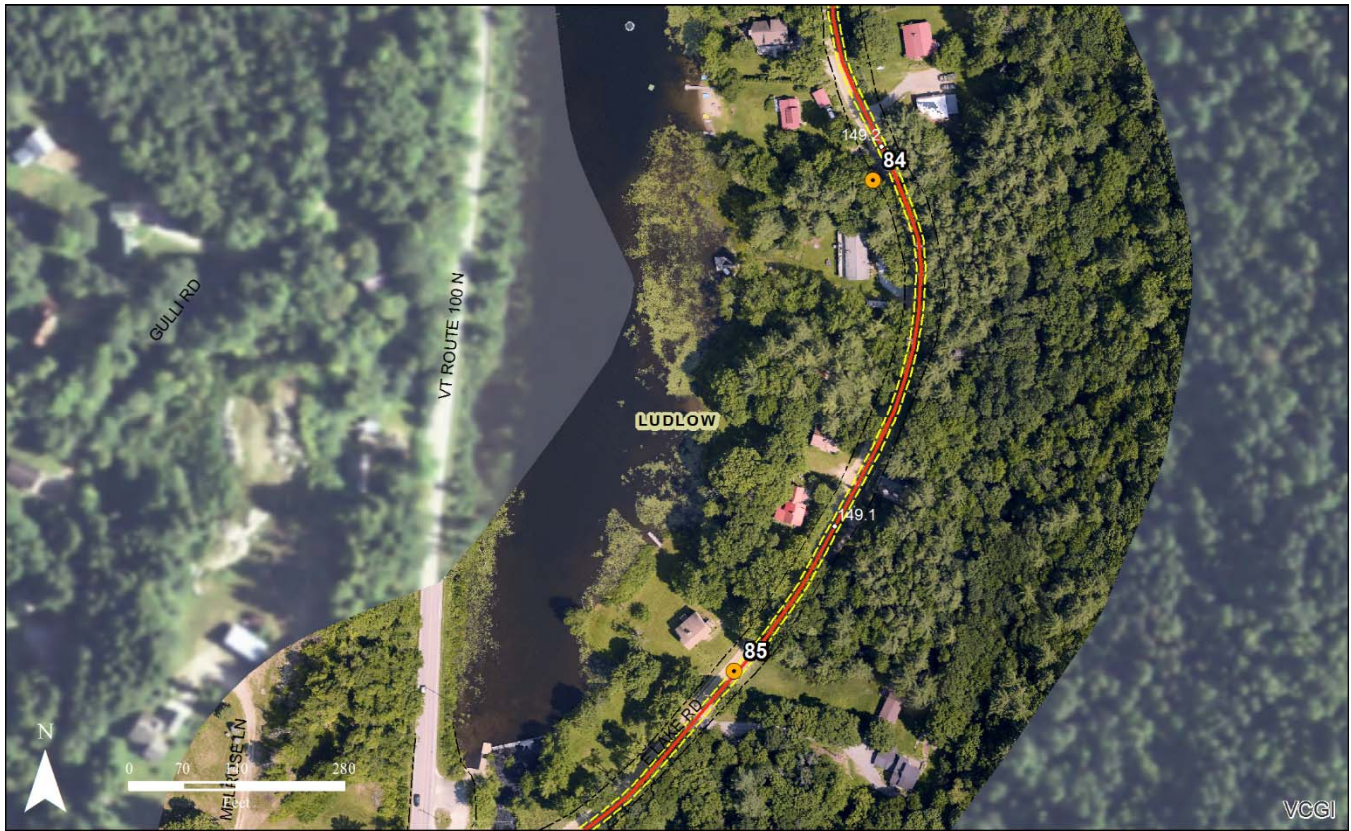
Assessment Map 50: After the line leaves Vermont Route 100, it will navigate a short series of dirt surfaced, class 3 town roads before terminating at the proposed converter station. The line will be buried beneath the road surface and generally, there will not be any clearing of vegetation along the side of these roads. Viewpoint 84 is on East Lake Road.
