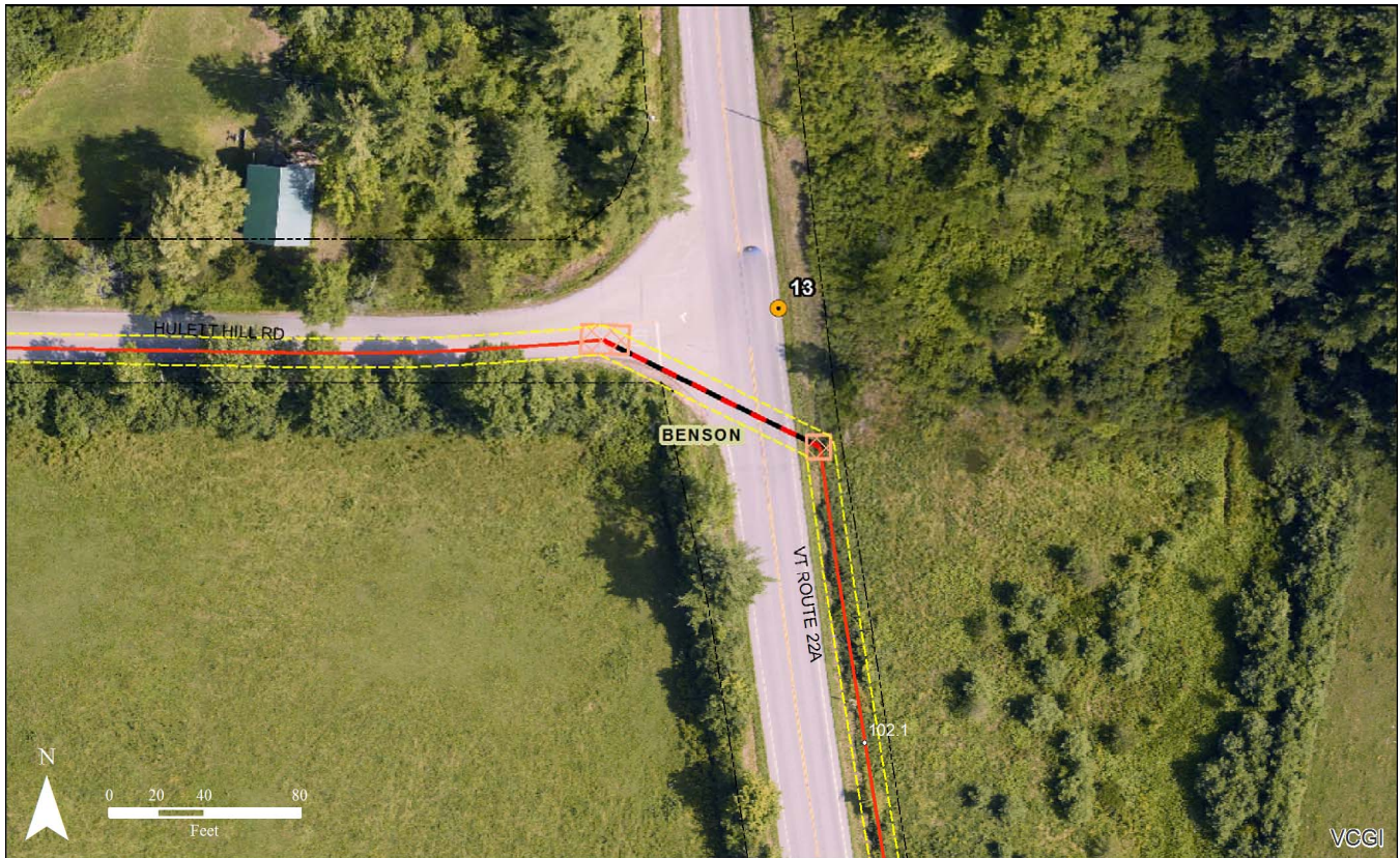
Assessment Map 10: At the east end of Hulett Hill Road, the Project will cross beneath Vermont Route 22A, angle south and run along the outside of the eastern shoulder of the road.
