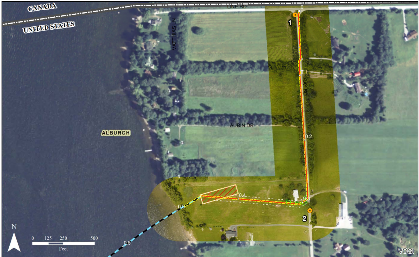
Assessment Map 1: The NECPL will run beneath the road surface for the first 400 feet along Bay road before shifting to just outside the western edge of the road. Vegetation along the west side of the road should be protected during construction.
