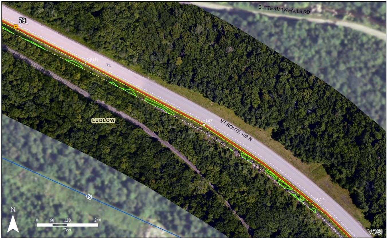
Assessment Map 46: In Ludlow, the line runs along the south/west side of the road and is typically located very close to the paved shoulder and will result in minimal clearing of roadside vegetation.
