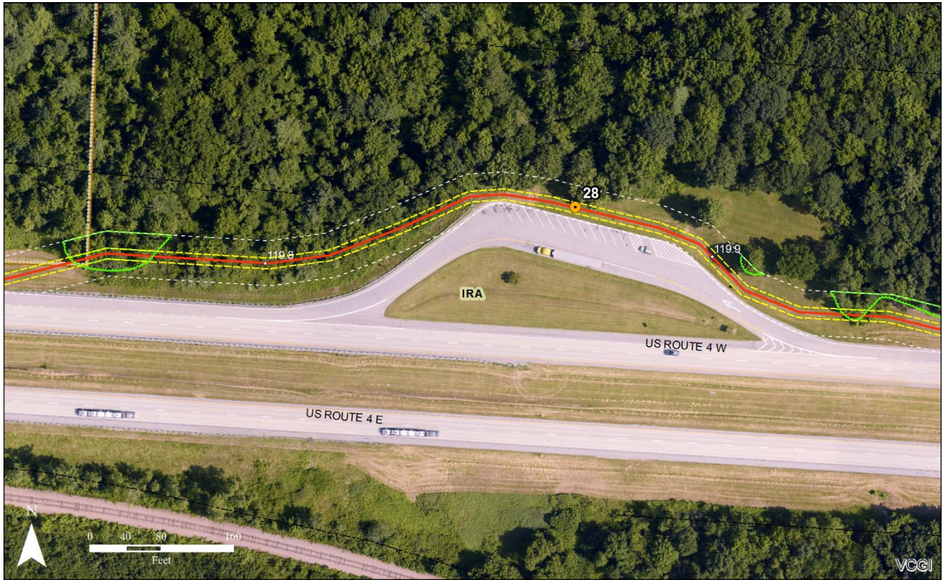
Assessment Map 24: At the west end of the pull-off along the westbound lanes of US Route 4, a 50-foot wide clearing will be necessary to allow construction of the Project.
