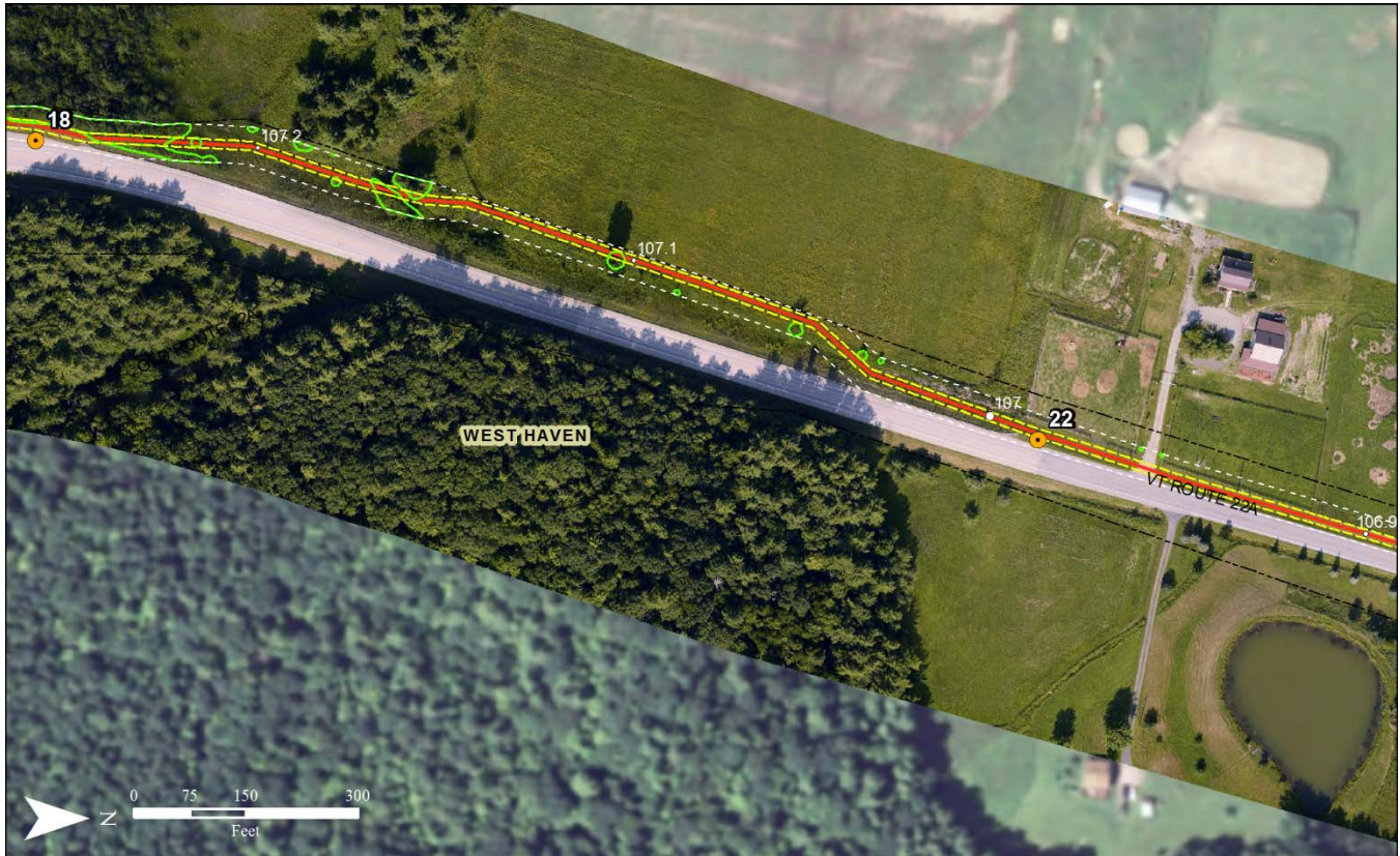
Assessment Map 15: As the route approaches MP 106.9 the line will diverge to the base of a highway embankment, along the outside of the right-of-way and will result in some minor vegetation removal on the embankment.
