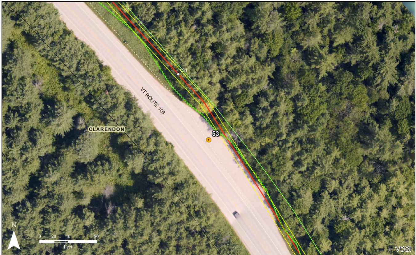
Assessment Map 33: At the intersection with Vermont Route 103, the Project turns east and continues along Vermont Route 103. Near MP 131.0, the line will be installed away from the edge of the road and clearing will be required up to the edge of the ROW, relocating the edge of woods up to 26 feet further from the road.
