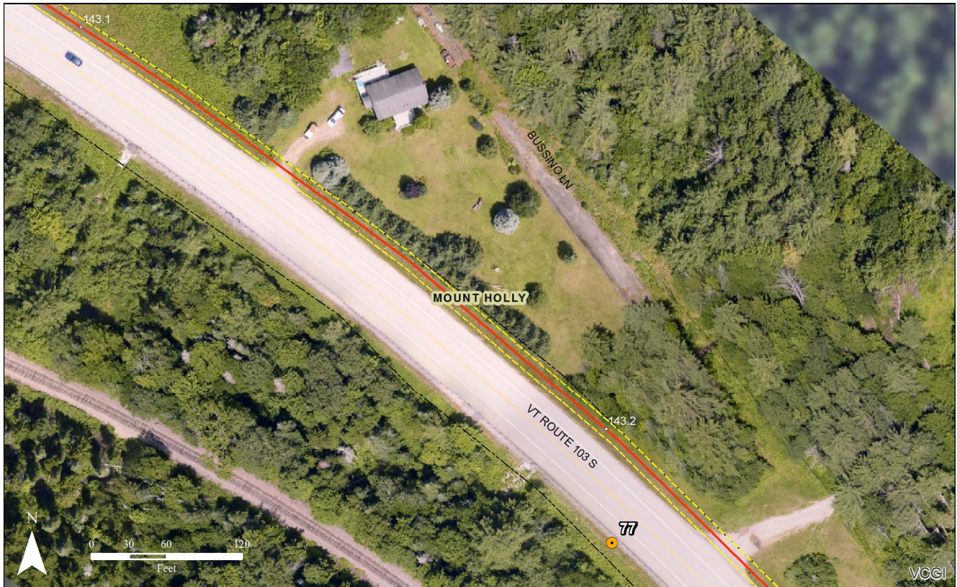
Assessment Map 45: Further east along Vermont Route 103. This location is an example of where the line will not require removal of the adjacent line of evergreen trees, but construction could damage the roots within the critical root zone of the tree.
