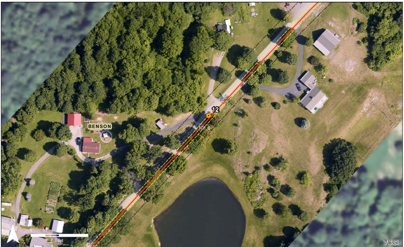
Assessment Map 9: From Stage Road, the Project route will connect to Vermont Route 22A via Hulett Hill Road. Similar to Stage Road, the line will be installed beneath the paved road surface for the length of Hulett Hill Road.
