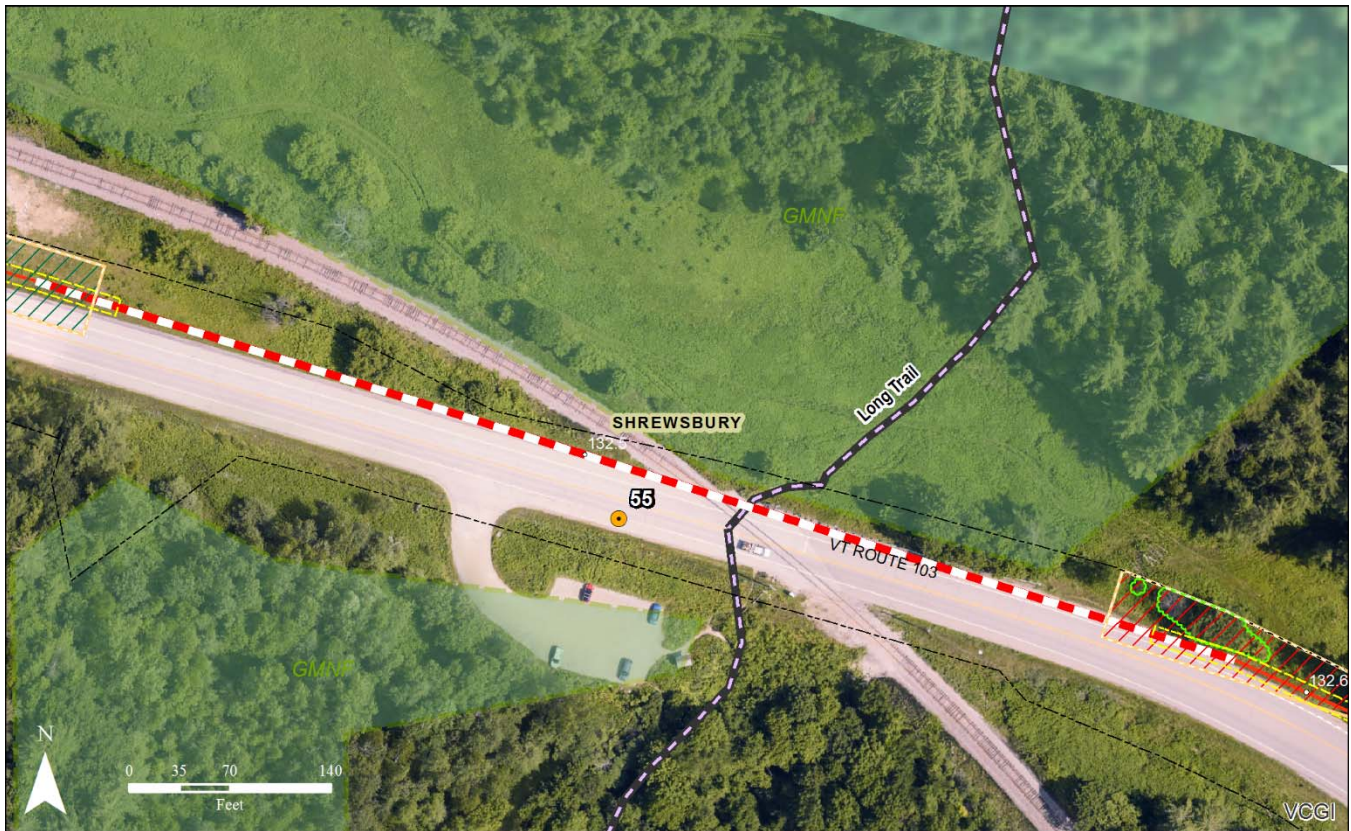
Assessment Map 35: At the Long Trail / Appalachian Trail crossing on VT Route 103, the line will be installed by HDD. Some limited clearing of shrubs and individual trees will be necessary at the eastern HDD staging area.
