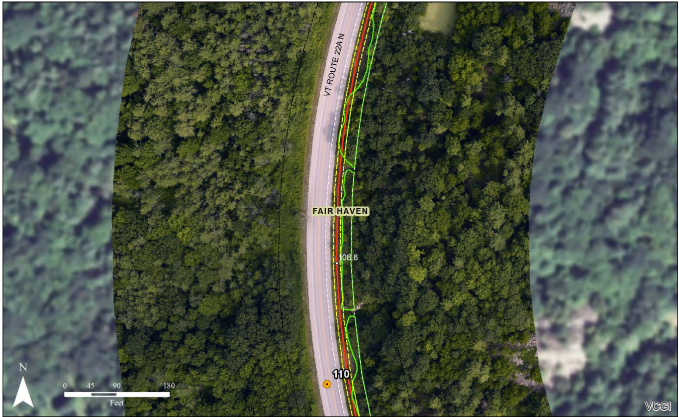
Assessment Map 16: From West Haven, the line continues into Fair Haven along the eastern side of Vermont Route 22A. Near MP 108.6, ledge may need to be removed along the edge of the roadway to install the cable.
