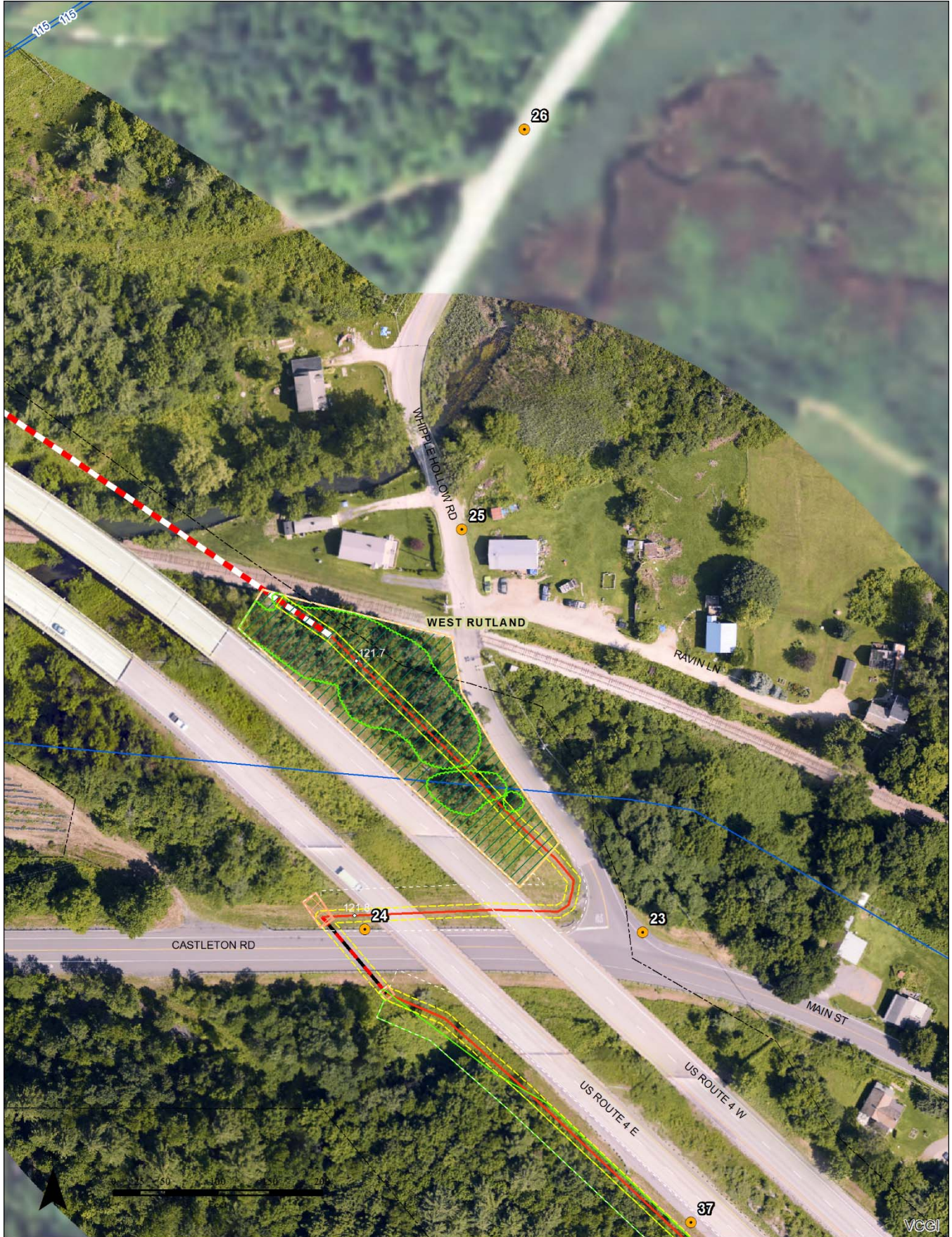
Assessment Map 25: The Project Route will be horizontally drilled beneath the Castleton River and then transition to the southern edge of the eastbound lanes of US Route 4 at the Vermont 4A (Main Street/Castleton Road) underpass.
