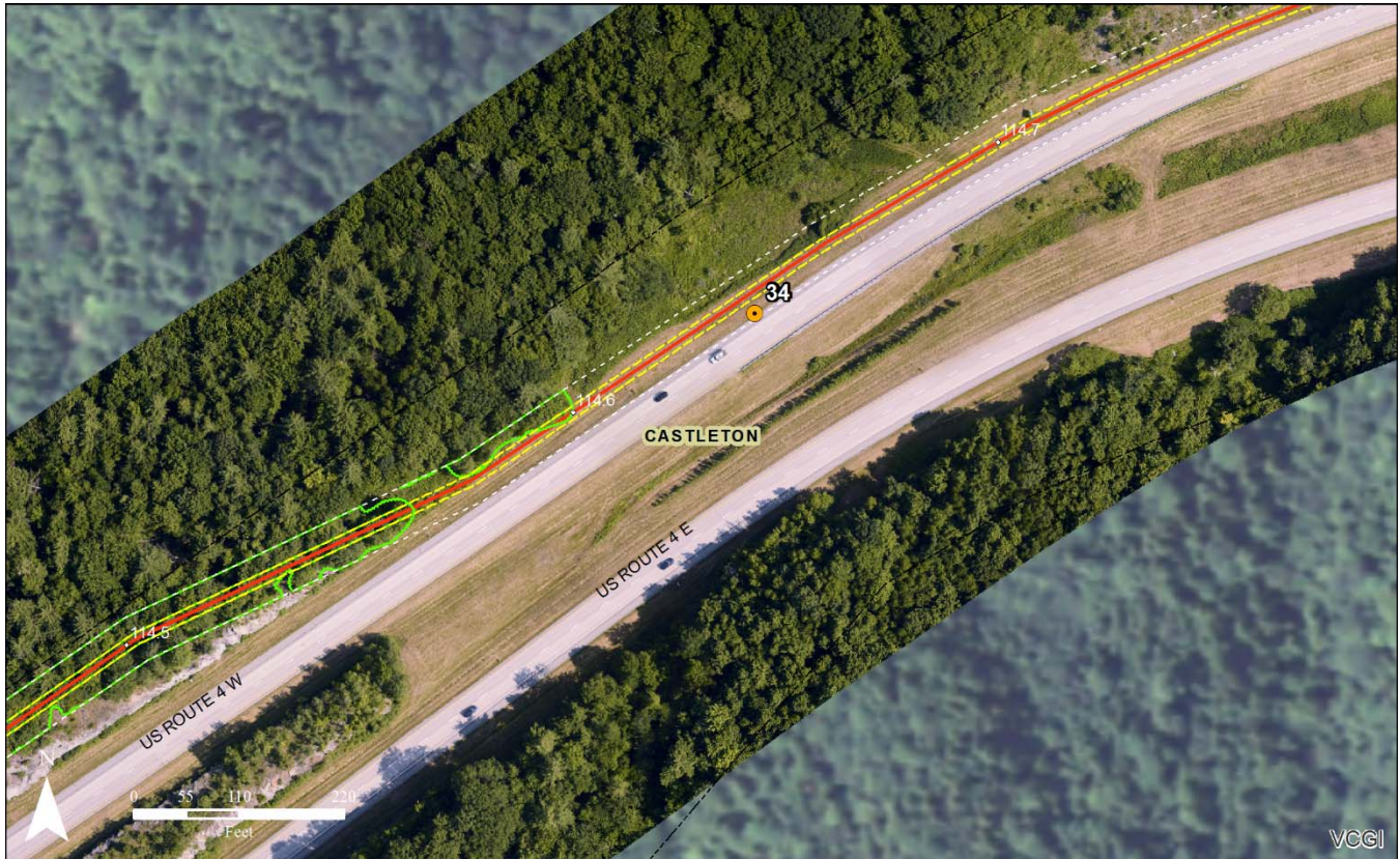
Assessment Map 20: Traveling westbound on US Route 4, this example shows one of the few locations where the line will be located above the top of a highway rock cut. Up to 50 feet of vegetation will be cleared from along the top of the rock cut, back towards the edge of the ROW to the north.
