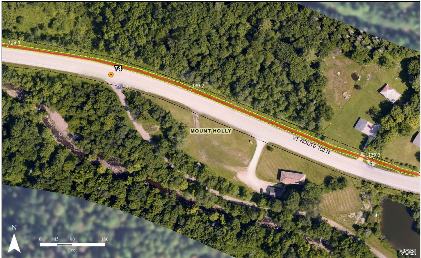
Assessment Map 42: The Project continues along Vermont Route 103 into Mount Holly. The area near MP 139.2 shows a typical location where the line will be installed within the existing clearing alongside the road.
