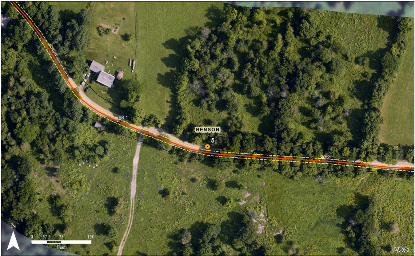
Assessment Map 3: Traveling south along the Project route, Stoney Point Road turns into North Lake Road, a similar dirt surfaced Class 3 Town Highway. The Project will be buried beneath the road surface and construction will not require removal of vegetation along the roadside.
