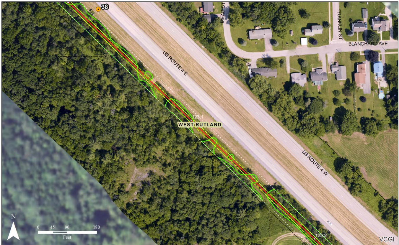
Assessment Map 26: Near MP 123, up to 50 feet of clearing from the bottom of the highway embankment towards the edge of the US Route 4 ROW is planned at this location.
