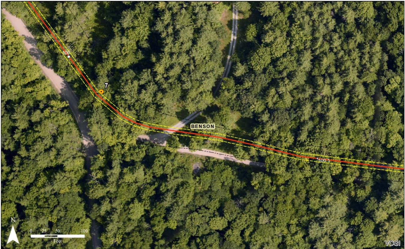
Assessment Map 5: Continuing southeast along North Lake Road from the intersection with Frazier Hill Road, the Project Route turns east onto Glenn Road, also known as Old North Lake Road. Glenn Road is a class 4 roadway and is only one lane wide at many locations with mature trees immediately adjacent to the road edge.
