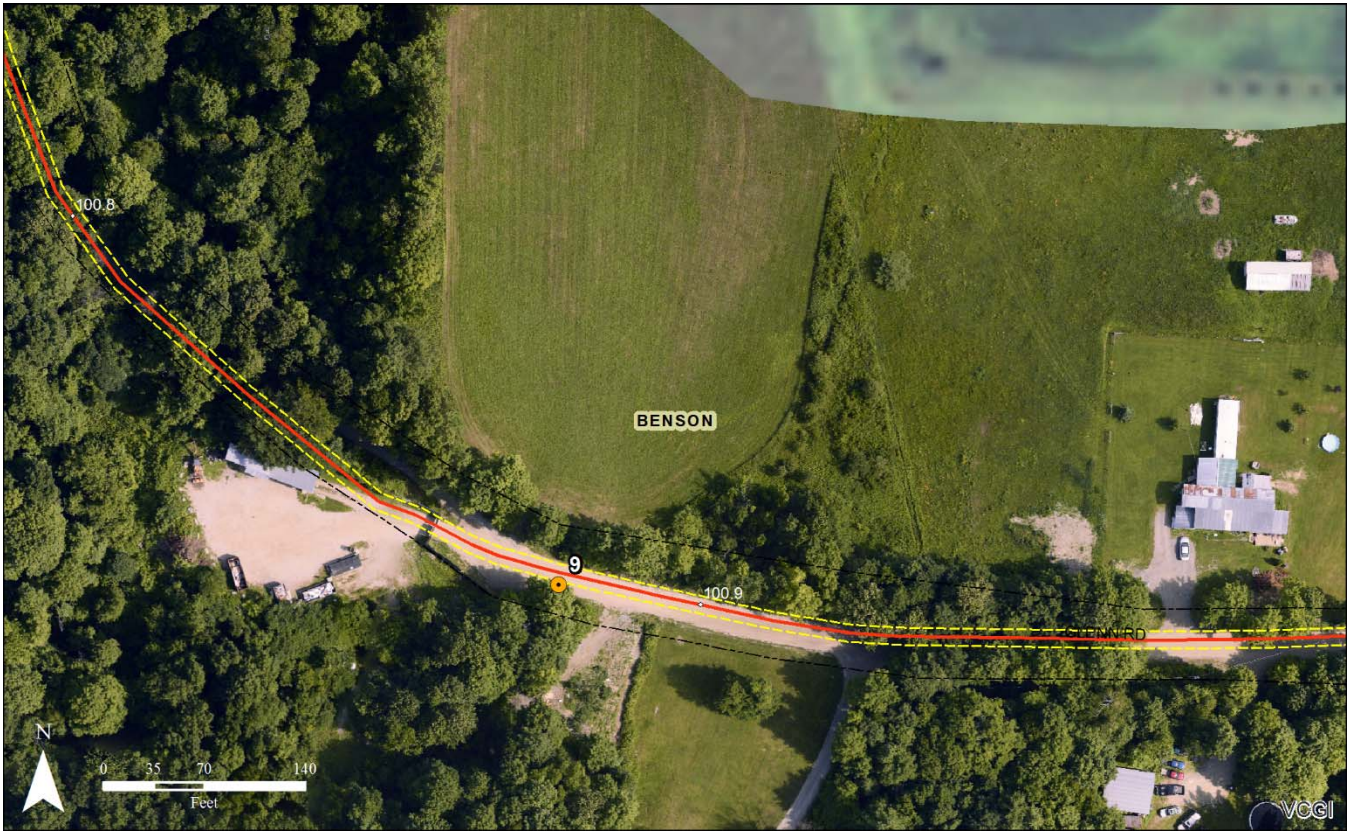
Assessment Map 7: Glenn Road (Old North Lake Road) at the Benson Transfer Station where the road classification changes from Class 4 (to the west) to Class 3 (to the east).
