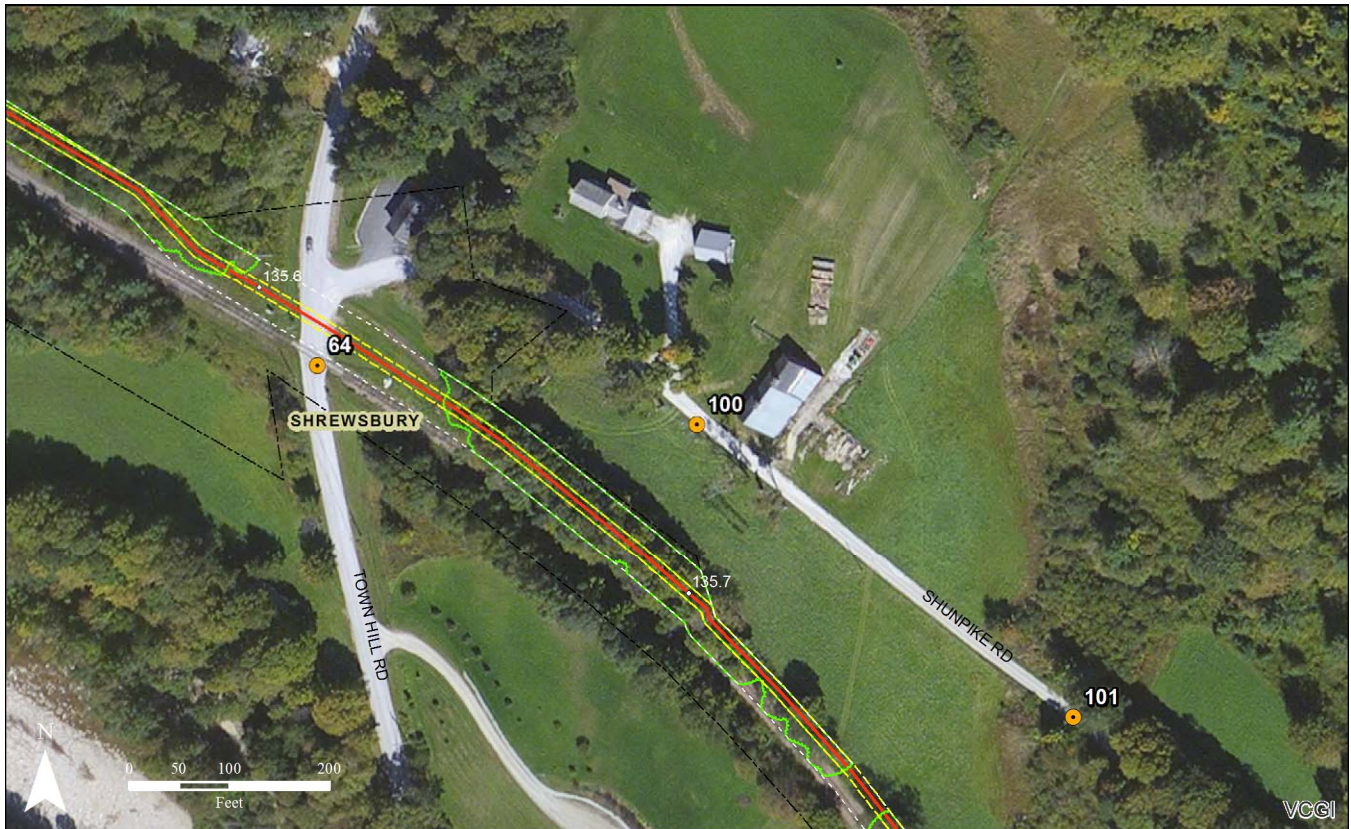
Assessment Map 38: At Town Hill Road, the line will be located to the northeast of the tracks and will require clearing up to 40 feet from the edge of the tracks.
